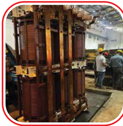
FURNACE TRANSFORMER (6.3 MVA 33KV/ 0.570KV-BSRM)
